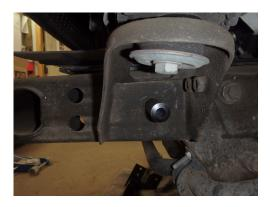
6.) Hold the receiver up in place and insert (6) 1/2" x 4 1/2" bolts with flat washers. Attach the plates on the inside of the frame with 1/2" flat washers and lock nuts. (NOTE: on 1500 models you may need to mark and drill the forward holes using a 1/2" drill bit).
